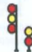
Proceed, medium speed passing signal and through turnouts, preparing to stop at next signal.
